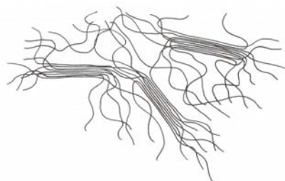
FIGURE 3.15. Schematic representation of a polymer matrix showing crystalline regions (fringed micelle model).
